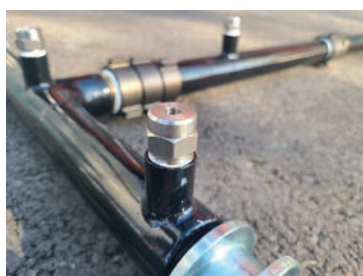
Fitted with mist cooling nozzles
